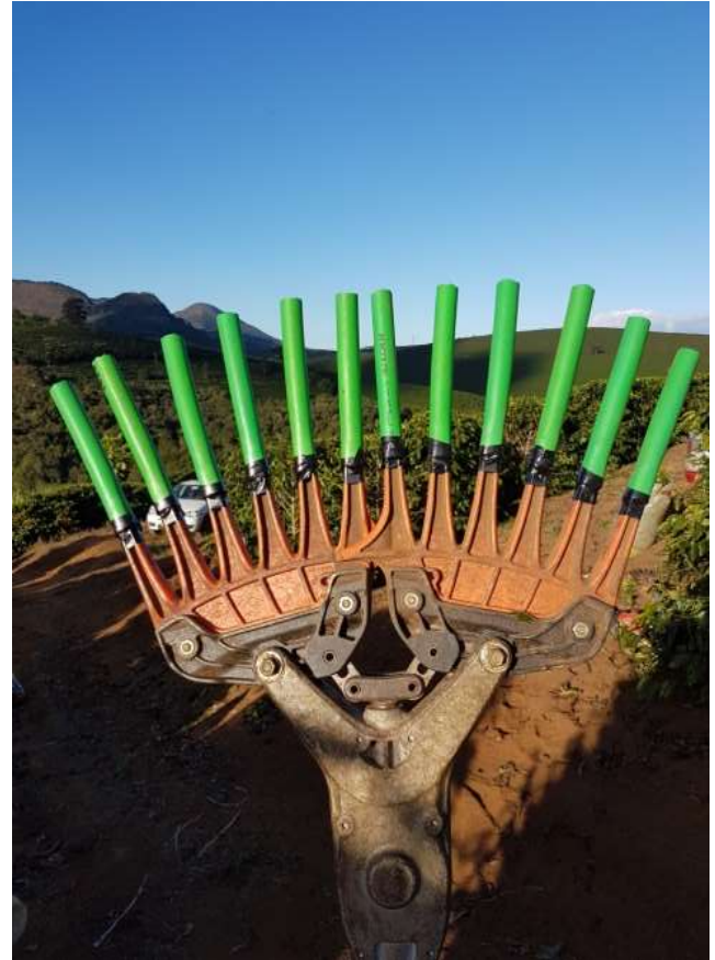
Figure 1. Flexible extenders placed at the tip of the portable derriere rods.
